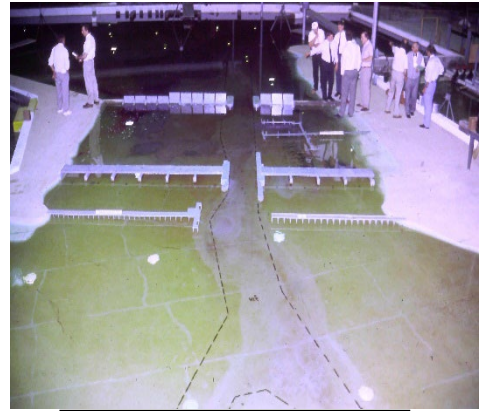
FLOODGATE PHYSICAL MODEL
